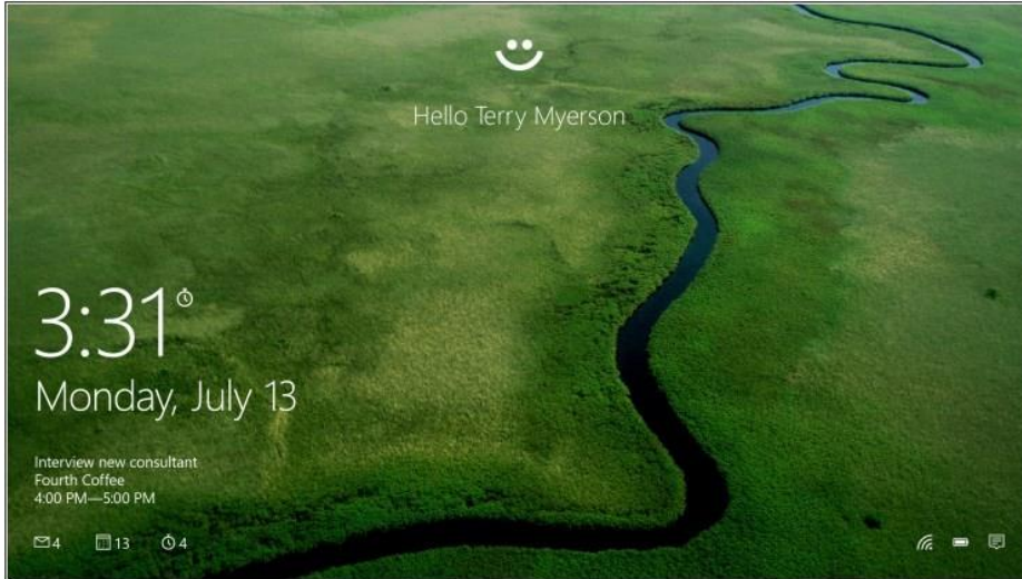
FIGURE 4-4 On consumer devices, biometric authentication allows local sign-in using a feature called Windows Hello.
